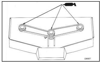
Figure 9. Spindle Lubrication
